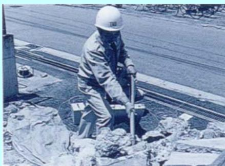
3. Adjust (automatically/manually) the level of radio wave emission and reception to conduct a search. Received radio waves will be displayed on the screen, as shown right, and sound corresponding to a wave pattern there is a survivor wave pattern will come out of the headset. The presence or absence of a survivor can be determined from both the wave shape and sound.
